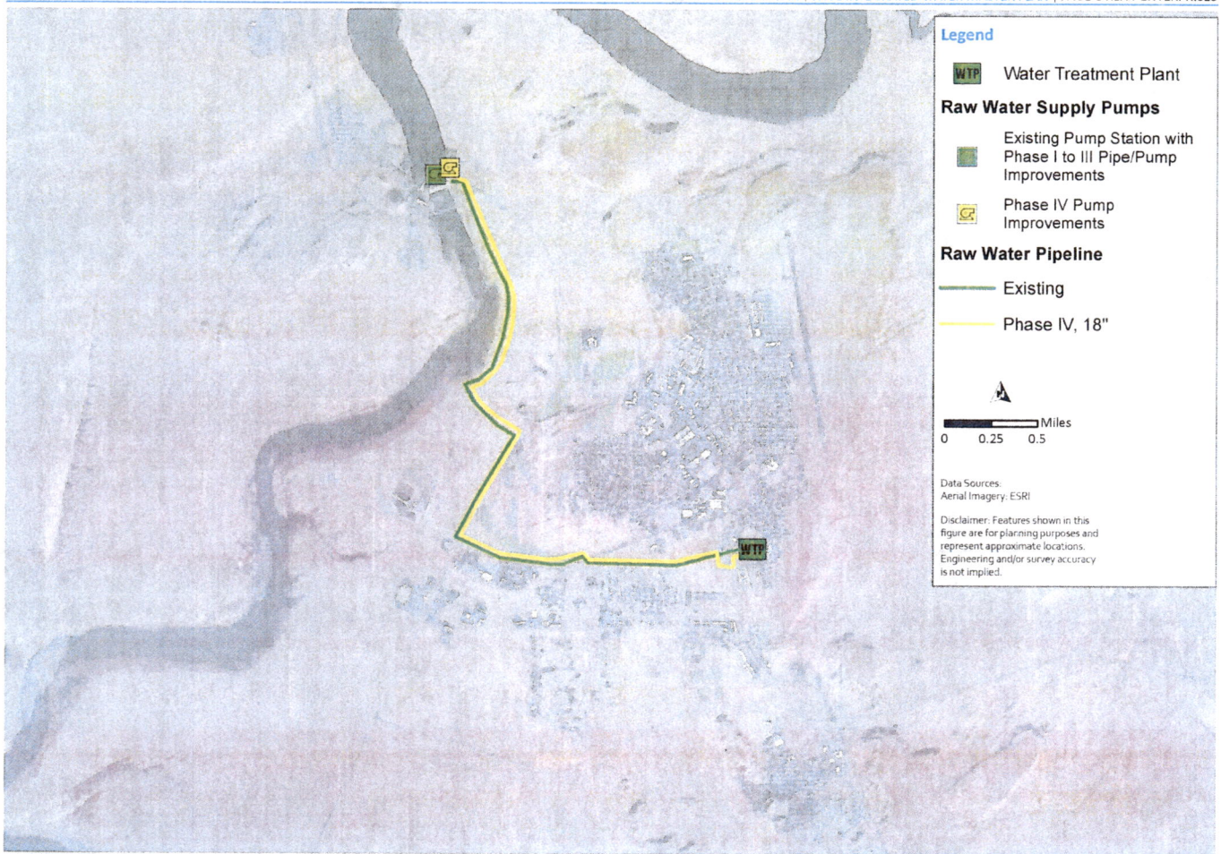
Figure 2.12 Option 1 Phased Raw Water System Improvements
